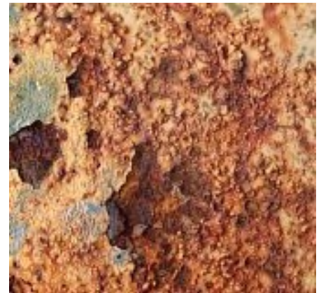
A close view of strong rust due to salt corrosion
